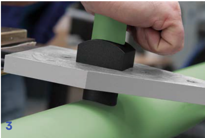
3. Welding the pipe saddle fitting by heating up the weld in saddle and use proper die.
